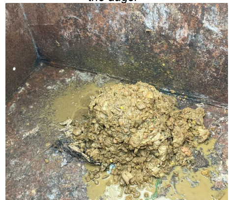
Material in dumpster direct from the auger without dewatering
