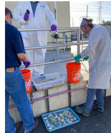
Rinsing screenings, removing organics, placing samples greater than 1 inch on blue tray for identification
