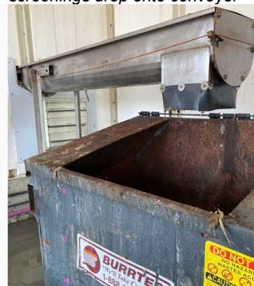
Compactor removed delivering direct from auger
